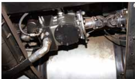
The MISER hybrid hydraulic transmission installed in the International truck.
